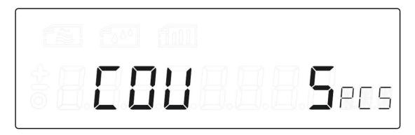
3. Press "ON" to select the quantity and put the corresponding quantity of samples. Press "O/T" to confirm and "COU --- PCS" will be displayed.
