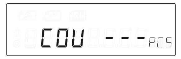
4. The operation can be started when the "COU ---" disappears and the corresponding number appears.
