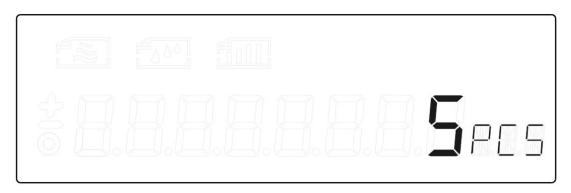
5. After the test is finished, press "ON" to select "weight", and press "O/T" to confirm to exit and return to the weighing interface.
