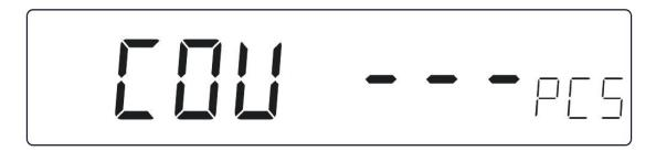
4. The operation can be started when the "COU ---" disappears and the corresponding number appears.
