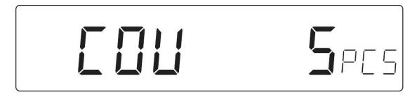
3. Press "UNIT" to select the quantity and put the corresponding quantity of samples. Press "TARE" to confirm and "COU --- PCS" will be
