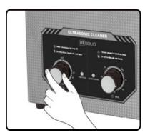
6. Heating is an optional function of the machine. Rotate the left knob clockwise/anticlockwise to increase/decrease the setting temperature. The heater indicator goes off when the actual temperature reaches the set temperature.
