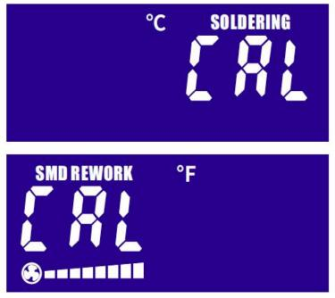
2. Press the hot air (soldering station) temperature increase or decrease button to enter the measured temperature value.
