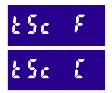
3. Press the soldering station temperature increase or decrease button to select either the Celsius or Fahrenheit display mode. Once done, press the hot air rework station temperature increase button to confirm setting and exit the setting interface.
