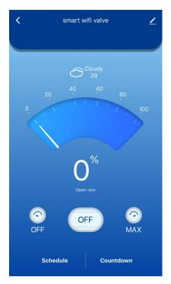
12. Tap "OFF" on the left side. The valve will close completely.
