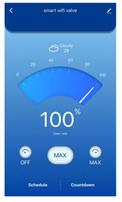
13. Tap "MAX" on the right side. The valve will open completely.
