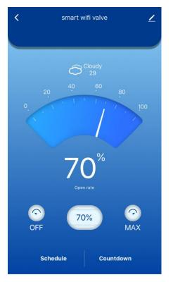
18. The smart valve will open or close to the selected open rate when the scheduled time is up.
