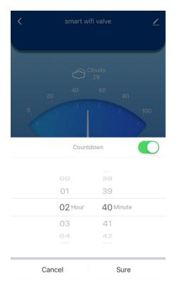
22. When the smart valve is open, tap the "Countdown" to set a time.
