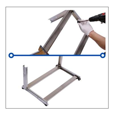
Install the non-slip feet to the bottom of the stand.
