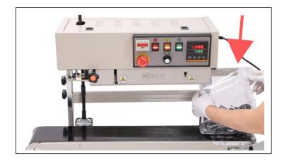
After setting the parameters of the control panel, the bag can be placed under the baffle to start the conveyor belt and begin the sealing process.
