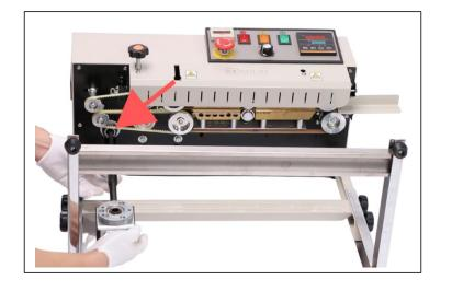
After connecting the bracket to the machine, place the machine down on the ground with the control panel of the machine facing up.
