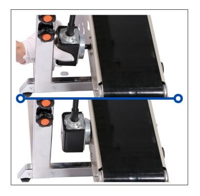
Insert the lever into the round hole in the transfer table.
