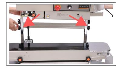
The yellow and black fasteners on both sides of the bracket can be used to adjust the height. Use both fasteners simultaneously to achieve the height needed for the bag you plan to seal.
