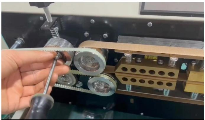
We have prepared a letter wheel for you which can be found in the accessory bag. This wheel can print numbers or letters onto the bag. You can use the small steel plate to unscrew the letter wheel and put the required letters into the letter wheel. Next, open the casing of the machine, remove the blank letter wheel with a screwdriver, and install the letter wheel you set.
