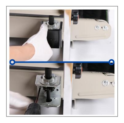
Take the black cover off the joystick. Using the screws provided, connect the joystick to the console.
