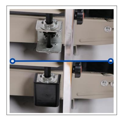
After tightening the screws, re-attach the black cover.
