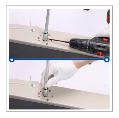
Remove the connecting rod screw on the side of the transfer table. This will allow you to release and remove the connecting rod.
