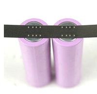
Check the welding effect
