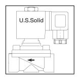
Note the directional arrow on your valve (located at the bottom). Most U.S. Solid valves are unidirectional, meaning they are designed for flow in one direction only, as shown in the figure on the left. If connected in the opposite direction, the valve will not actuate properly (normally closed valves will not close). Additionally, ensure the medium flowing through the valve is filtered; otherwise, particles may cling to the gasket over time and prevent proper sealing.
