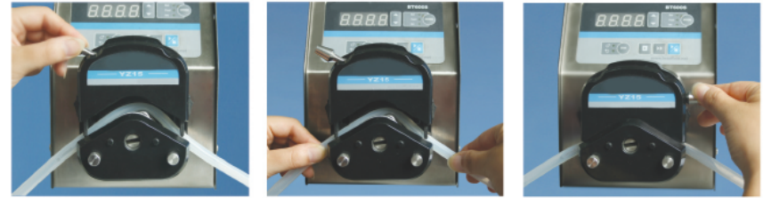
Figure 4 Example Diagram of Tube Installation Process
