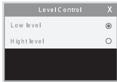
Figure 31 Level Signal Interface
