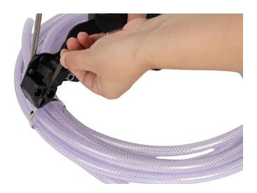
4. When the strap is tightened, the left-hand pulls up the cutter to cut it off, and the strap is cut off and moved away from the cutter so that a stainless steel band is installed.
