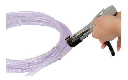
4. When the strap is tightened, Grip the handle tightly and cut the cable tie.
