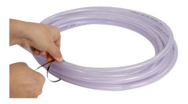
3. Insert the end of the binding band into the cutter. Hold the cutter's handle in your right hand and repeat the clenching until the binding band is tightened.
