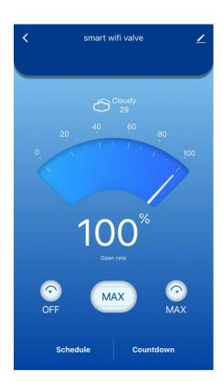
13. Tap "MAX" on the right side. The valve will open completely.
