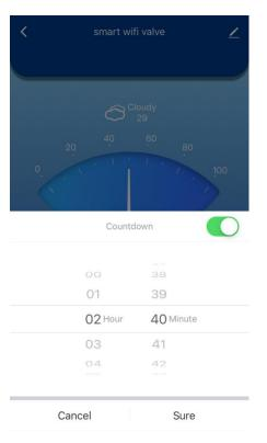
22. When the smart valve is open, tap the "Countdown" to set a time.
