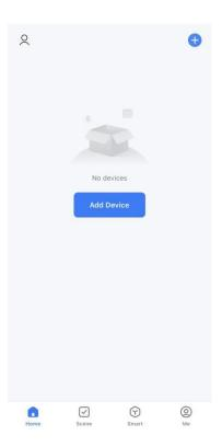
2. After connecting the U.S. Solid Smart Valve to the power, tap "Add Device" or the "+" at the upper-right corner.
