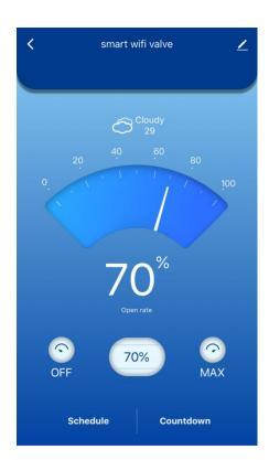
18. The smart valve will open or close to the selected open rate when the scheduled time is up.
