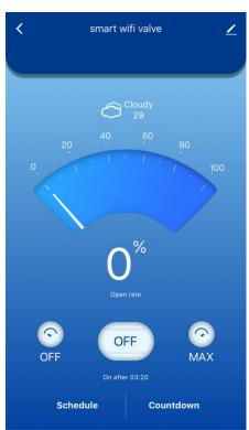
20. The smart valve will automatically open to max when the countdown is over.
