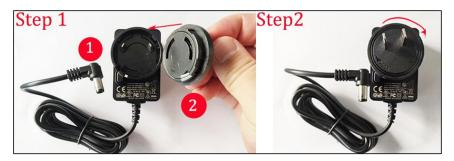
The power cord and plug are packaged separately. Please assemble them as shown in the figure above. Install part (2) onto part (1), then press part (2) down and rotate it anticlockwise.
