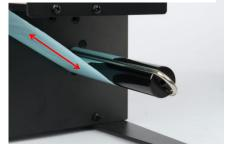
6.Grip the label end to the rewinding shaft and secure it with the U Pin, ensuring that the label paper is straight.
