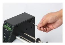
1.Unscrew the screw using the L tool.
