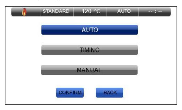
7. If timing ending mode is selected, then it is needed to click "TIME SETTING" icon to set a drying time. Use "^" or "V" to select required drying time and confirm by clicking "CONFIRM".
