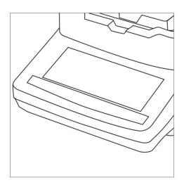
Wipe the panel with a damp cloth. Do not use a chemical dust cloth, as it may damage the paint surface and display panel.
