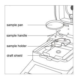
Remove sample pan, sample handle, sample holder and draft shield for cleaning. Ensure that no liquid seeps into the device. Dry with a dry soft cloth after cleaning.
