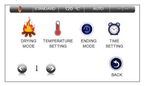
4. Click the "DRYING MODE" icon to select the required drying mode and confirm by clicking "CONFIRM".
