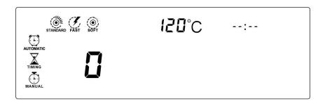
2. Use the "UP" or "DOWN" buttons to select desired serial number of a method and confirm it by pressing the "CONFIRM" button. The icon of the currently set drying mode flashes.
