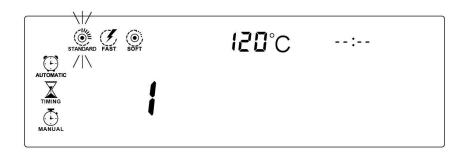
Press the "UP" or "DOWN" to select the required drying mode and confirm by pressing "CONFIRM".
