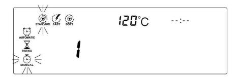
After drying mode is set, the icons for ending mode and the currently set drying mode flashes. Press the "UP" or "DOWN" to select required ending mode and confirm by pressing "CONFIRM".
