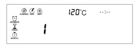
3. Confirm by pressing the "CONFIRM" button, the drying mode flashes.
