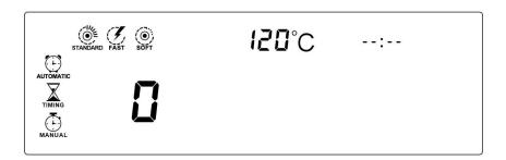
2. Press the "UP" or "DOWN" to select the number, where "0" is the factory setting (can't be changed) and "1" - "F" is the adjustable setting.
