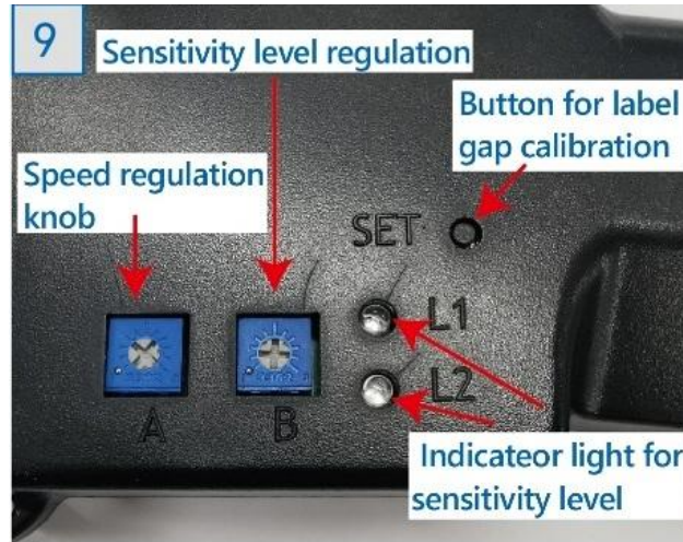
Speed knob, sensitivity knob, calibration button, and L1/L2 sensitivity indicators.
