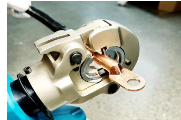
6. Place the terminal in the die groove.
