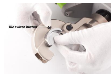
3. Press the switch on the other side and place another die in the center position.
