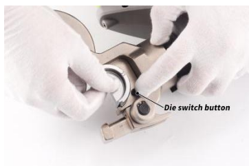
2. Press the die switch button and place the die in the center position.
