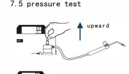
Close the flame torch, and gas pressure will become higher and higher.When it reaches its limit, current value will become zero, and machine will stop work. Then lift the pressure-releasing valve, there will be gas releasing.In that case, the machine works well.
