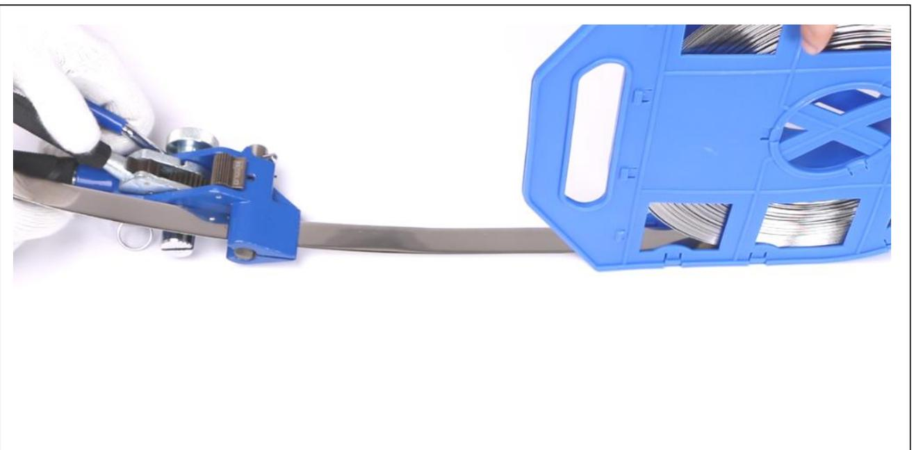
② Insert the band through the seal with the ears facing up. Then, bend the end of the band under the seal. Insert the other end of the stainless steel strap into the packing buckle.
