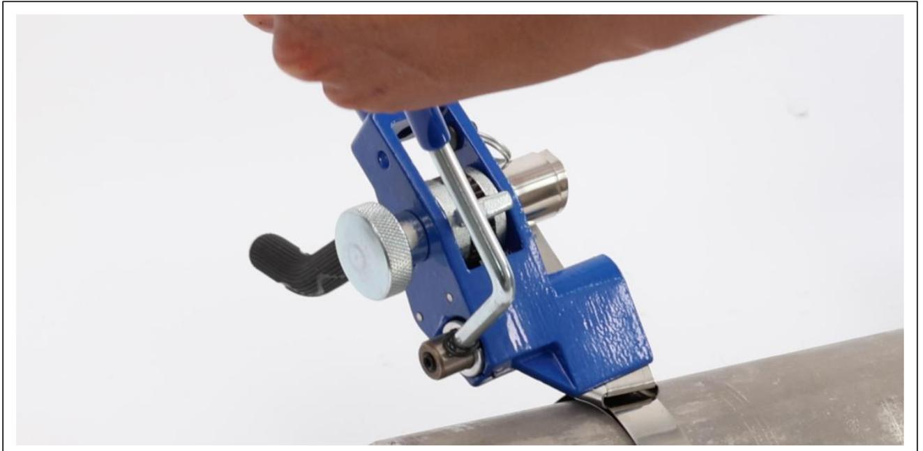
⑧ Knock the stainless steel belt into the packing buckle with a hammer, and then use a hammer to hit the ears of the packing buckle to both sides of the stainless steel belt to fix the packing buckle.
