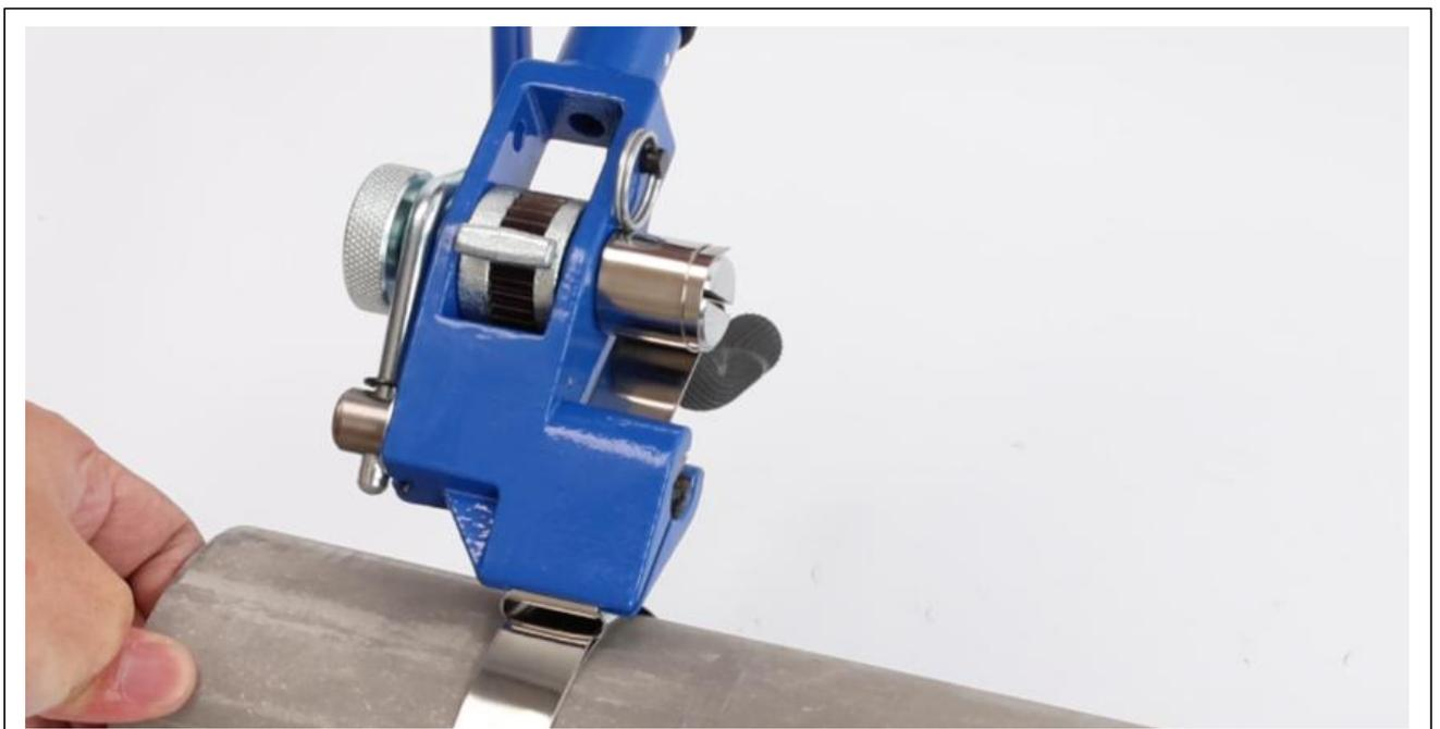
⑦ Hold the black handle tightly with your left hand, and the blue handle with your right hand, pull the two handles in opposite directions and cut off the stainless steel strapping.
