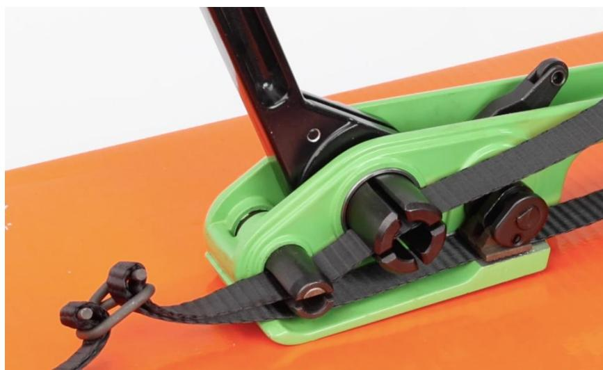
3. While holding the tool with your left hand, push and pull the handle back and forth with your right hand until the packing strapping is tightened.
