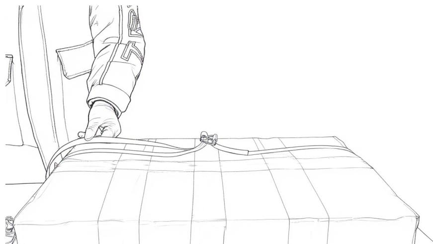
2. As shown in the picture, place the lower packing strapping under the lower tooth plate and the cutter body, and slide the upper packing strapping tie into the cutter groove and the spindle groove.
