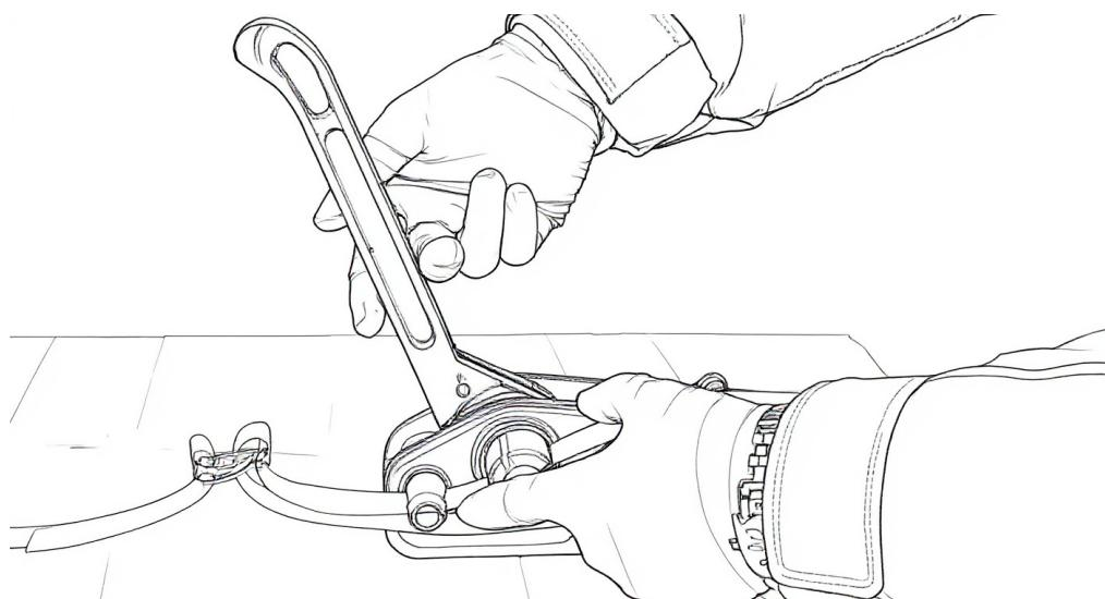
3. While holding the tool with your left hand, push and pull the handle back and forth with your right hand until the packing strapping is tightened.
