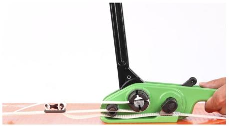
4. Press down on the handle of the tool with your right hand, and after cutting off the strapping, press the handle tool firmly to the right to remove it.
