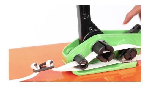
3. While holding the tool with your left hand, push and pull the handle back and forth with your right hand until the packing strapping is tightened.
