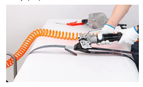
4. As shown in the following picture, position the locking machine on the steel buckle and press the switch handle to complete the locking process.
