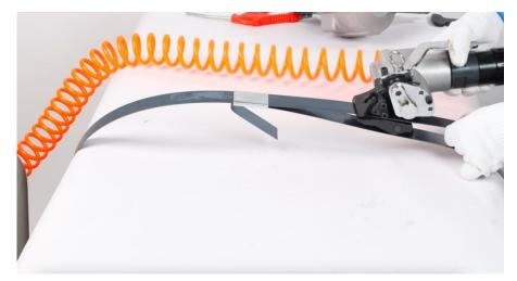
3. As illustrated in the subsequent image, the rotating ring at the end of the motor body has three positions: stop, half-open, and fully open. Rotate the ring clockwise. When the tensioning wheel turns, the steel belt tightens until it reaches a saturated state. At this point, it will cease rotating, yet the rotating ring will remain fixed in the fully open position.
