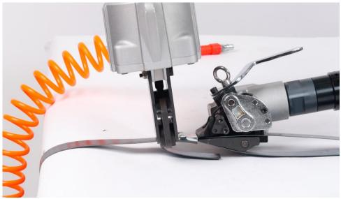
5. As shown in the following picture, after completing the locking action, tilt the tensioning machine upward to the vertical position until the steel strip breaks, and then turn the rotating ring to the stop position.
