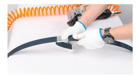
2. As illustrated in the following picture, grasp the motor body and press the handle with your thumb. Allow the steel belt, passing through the upper layer of the steel buckle, to be inserted between the tensioning wheel and the roller, then release the handle.
