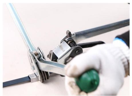
4. Use your thumb to press the pawl handle on the machine handle forward, and then squeeze the machine handle and the machine body together, so that the pressure wheel rises and the baler can be moved to the right.
