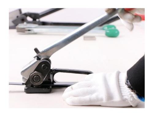
3. Place the strapping buckle on the iron belt and once the desired tension is reached, seal it with pliers.
