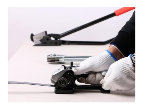
2. Swing the machine handle until the steel strap is tightened, and then press the machine handle to a lower position. (It is not recommended to press the machine handle to an extremely low position, otherwise, the pressing wheel will be lifted and the packing iron sheet will be loosened).
