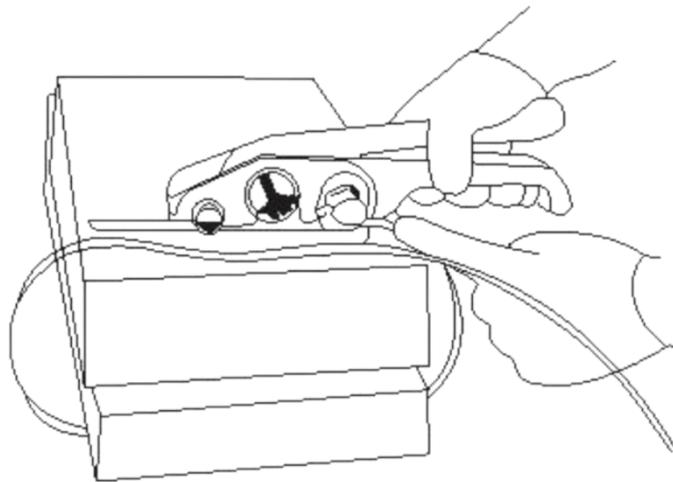
2. Slide the strapping into the cutter groove and spindle groove.
