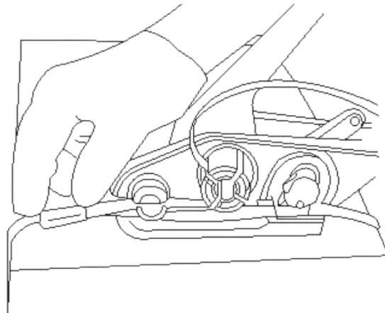
5. Place this sealer tool fully open over the buckle, then close the handle so that the buckle is fully clamped, then remove the sealer tool.
