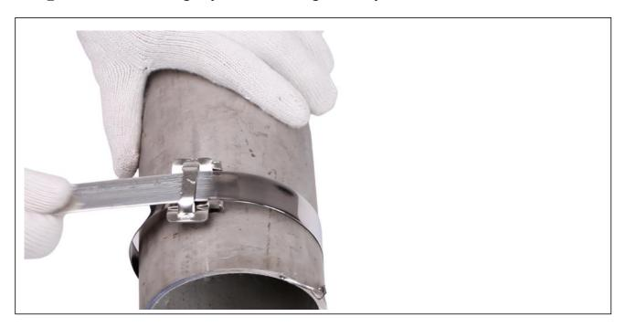
④ Hold the tool in your left hand as shown. Line up the slots in the nose and windlass so they are on a straight line. Insert the band through the nose and windlass slots.
