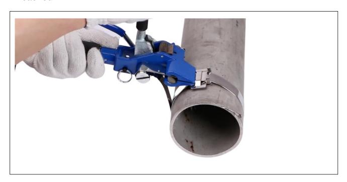
⑥ Place the tool on top of the goods in the direction shown in the figure.
