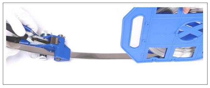
② Insert the band through the seal with the ears facing up. Then, bend the end of the band under the seal. Insert the other end of the stainless steel strap into the packing buckle.
