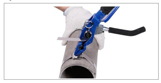
Thold the black handle tightly with your left hand, and the blue handle with your right hand, pull the two handles in opposite directions and cut off the stainless steel strapping.
