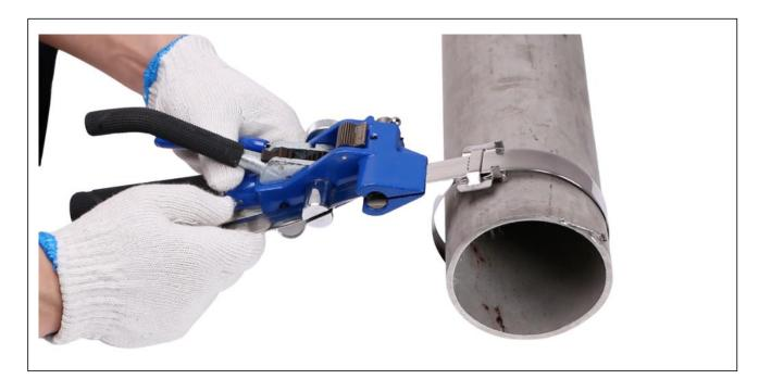
⑤ Hold the black rocker in your right hand in the position shown. Push the rocker forward and backward until the desired tension is reached.
