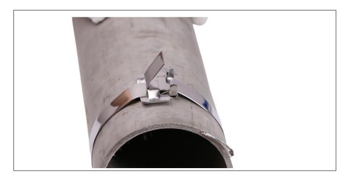
(7) Knock the stainless steel belt into the packing buckle with a hammer, and then use a hammer to hit the ears of the packing buckle to both sides of the stainless steel belt to fix the packing buckle.
