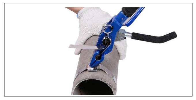
⑦ Hold the black handle tightly with your left hand, and the blue handle with your right hand, pull the two handles in opposite directions and cut off the stainless steel strapping.
