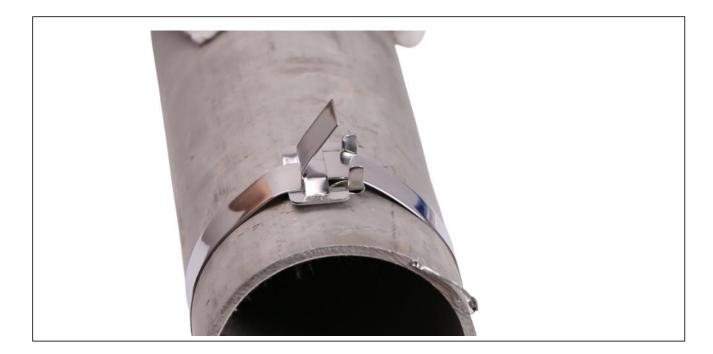
⑦ Knock the stainless steel belt into the packing buckle with a hammer, and then use a hammer to hit the ears of the packing buckle to both sides of the stainless steel belt to fix the packing buckle.
