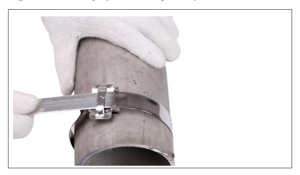
④ Hold the tool in your left hand as shown. Line up the slots in the nose and windlass so they are on a straight line. Insert the band through the nose and windlass slots.
