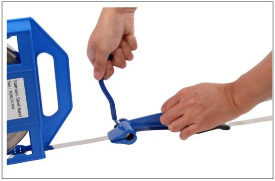
② Insert the band through the seal with the ears facing up. Then, bend the end of the band under the seal. Insert the other end of the stainless steel strap into the packing buckle.
