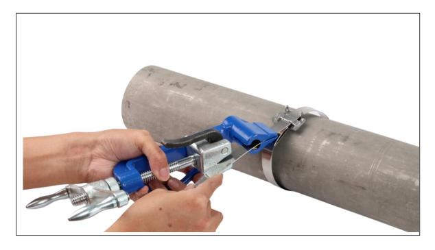
⑤ Hold the black rocker in your right hand in the position shown. Push the rocker forward and backward until the desired tension is reached.
