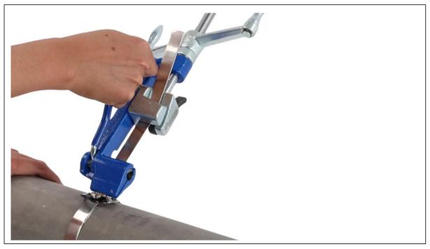
Thold the black handle tightly with your left hand, and the blue handle with your right hand, pull the two handles in opposite directions and cut off the stainless steel strapping.
