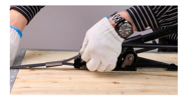
2.Insert the strapping into the cutter groove and spindle groove.
