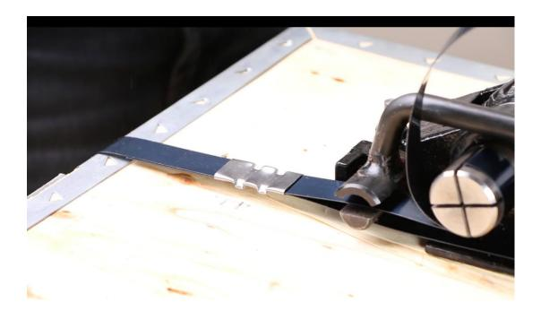
5. Press the handle of the tensioner to cut the strapping, and press the handle to move the tool to the right until it is removed from the strapping.
