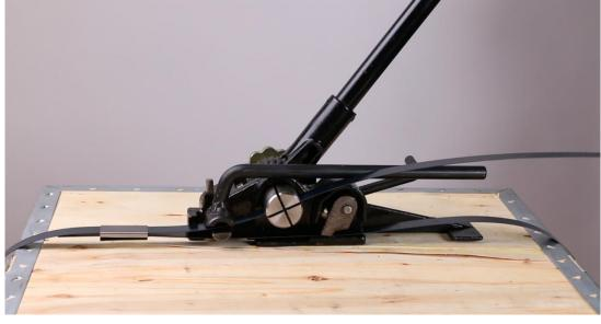
3. Swing the handle back and forth with your right hand until the strapping is pulled tight.
