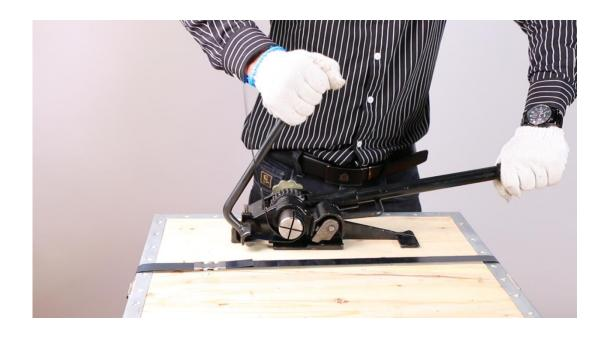
6.If you are not satisfied with the packaging, as shown in the picture, you can use the steel strip scissors we prepared for you to cut the steel strip.
