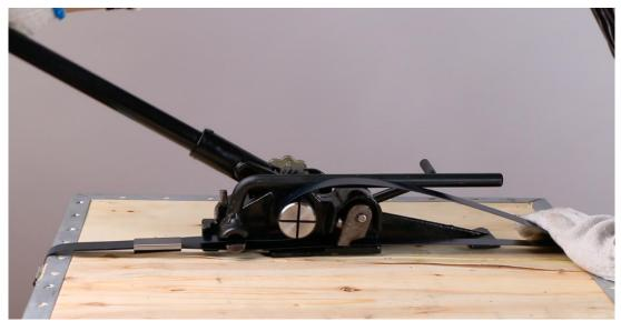
4. Place the sealer tool fully open over the buckle, then close the handle so that the buckle is fully clamped, then remove the sealer tool.
