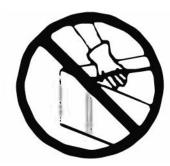
Do not put upir hands or other parts of the body between the strap and the package during the strapping process.
