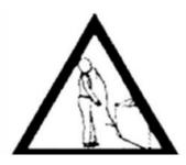
Do not stand in line with the strap while it is tensioned. The strap could break.
