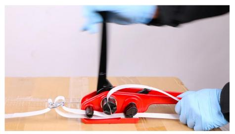
4. Press down on the handle of the tool with your right hand, and after cutting off the strapping, press the handle tool firmly to the right to remove it.
