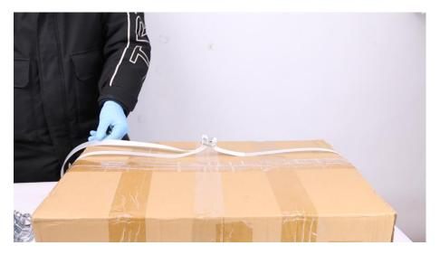
2. As shown in the picture, place the lower packing strapping under the lower tooth plate and the cutter body, and slide the upper packing strapping tie into the cutter groove and the spindle groove.
