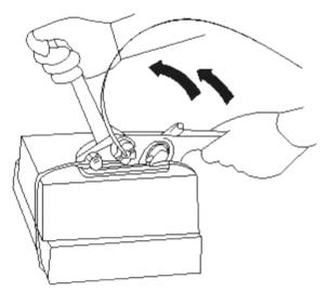
4. After pulling the strapping to the appropriate tightness, place the buckle with the opening facing down on the strapping.
