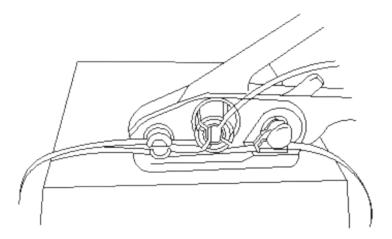
3. Hold the tensioner with your left hand and swing the handle back and forth with your right hand until the strapping is pulled tight.
