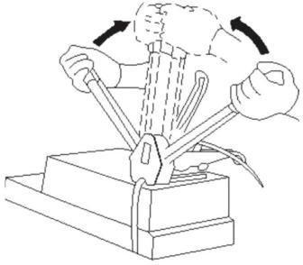
6. Press the handle of the tensioner to cut the strapping, and press the handle to move the tool to the right until it is removed from the strapping.
