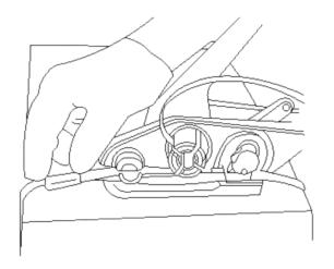
5. Place the sealer tool fully open over the buckle, then close the handle so that the buckle is fully clamped, then remove the sealer tool.
