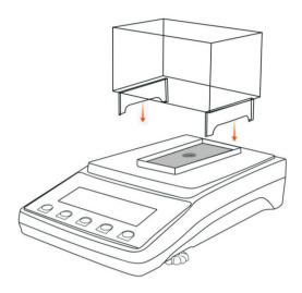
3. Place the bracket across the top of the container and the bottom of the bracket fits into both ends of the weighing pan;
