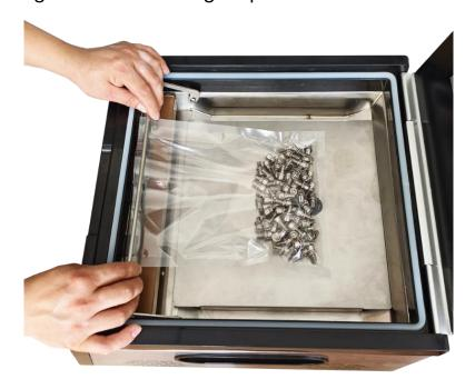
2. Press the front and edge of the vacuum hood, then start the vacuum process.
