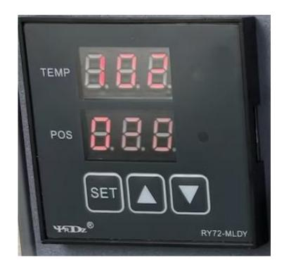
TEMP shows the set temperature of the ink wheel, and it is recommended to set it between 80-100. POS shows the position of the text. The larger the number is, the closer the text position is to the right side of the bag. (Adjust the appropriate position according to the width of the bag).
