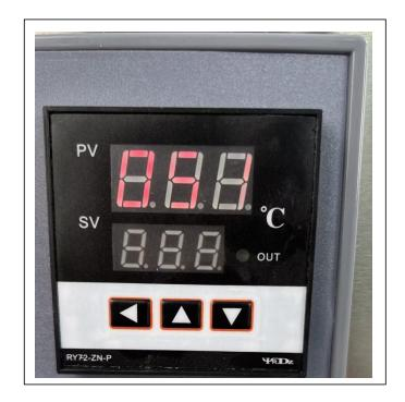
A. The number displayed by PV indicates the current actual temperature. The number next to SV indicates the temperature we set.
