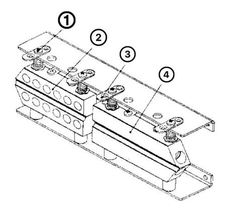
Adjustment of the distance between the upper and lower heating blocks and cooling blocks: Due to different sealing materials and their thickness, the distance between the upper and lower heating blocks and cooling blocks needs to be adjusted for each product that is sealed. This can be done by turning the upper adjustment screw ① to the left to reduce or increase the distance between the upper and lower heating blocks and the cooling block.
