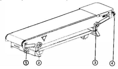
Conveyor belt tension adjustment: When the conveyor belt is too loose or too tight, turn the two "conveyor belt tension adjustment knobs" at the same time (right-handed for tension, left-handed for loosening) until the conveyor belt is tight enough.
