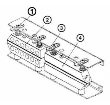
Adjustment of the distance between the upper and lower heating blocks and cooling blocks: Due to different sealing materials and their thickness, the distance between the upper and lower heating blocks and cooling blocks needs to be adjusted for each product that is sealed. This can be done by turning the upper adjustment screw C to the left to reduce or increase the distance between the upper and lower heating blocks and the cooling block.
