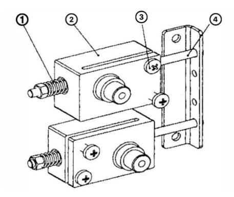
If the sealing belt runs sideways, it can be adjusted through the adjusting screw on the passive wheelbase ②.
