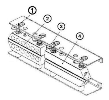
Adjustment of the distance between the upper and lower heating blocks and cooling blocks: Due to different sealing materials and their thickness, the distance between the upper and lower heating blocks and cooling blocks needs to be adjusted for each product that is sealed. This can be done by turning the upper adjustment screw C to the left to reduce or increase the distance between the upper and lower heating blocks and the cooling block.
