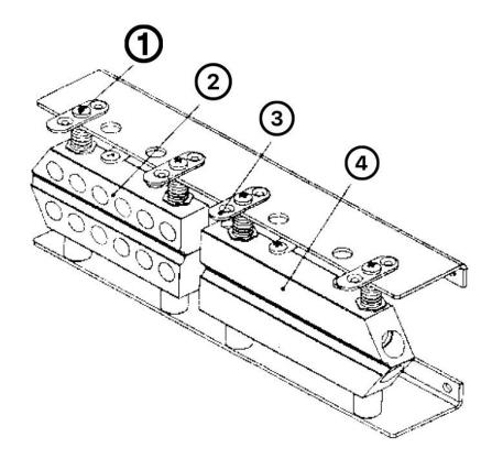
Adjustment of the distance between the upper and lower heating blocks and cooling blocks: Due to the different sealing materials and thicknesses, the distance between the upper and lower heating blocks and cooling blocks needs to be adjusted for each product seal. For the distance between the upper and lower heating blocks and the cooling block, turn the upper adjustment screw ① to the left to reduce the distance between the upper and
