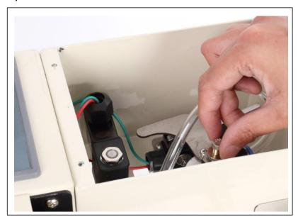
c). Take one piece of plastic bag, open its mouth, then put the gas nozzle into the plastic bags.
