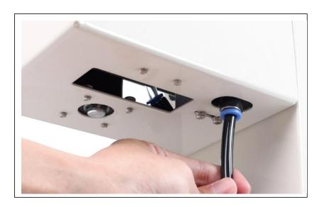
b). Adjust the air output: rotate counterclockwise to increase the output, or clockwise to decrease it.
