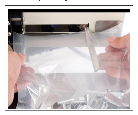
d). Put the plastic bags into the wheels, let the gas fill into the bag, then it will be conveyed and sealed.
