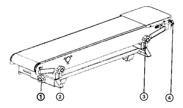
Conveyor belt tension adjustment: When the conveyor belt is too loose or too tight, turn the two "conveyor belt tension adjustment knobs ④" at the same time (right-handed for tension, left-handed for loosening) until the conveyor belt is tight enough When appropriate.
