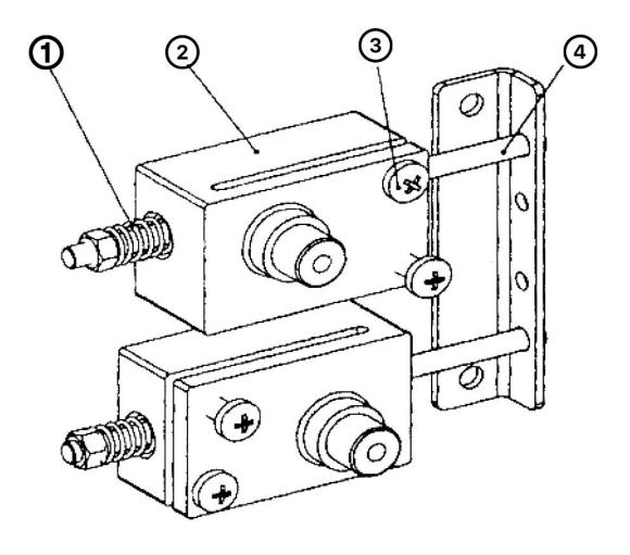
If the sealing belt runs sideways, it can be adjusted through the adjusting screw on the passive wheel base 2.
