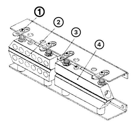
Adjustment of the distance between the upper and lower heating blocks and cooling blocks: Due to the different sealing materials and thicknesses, the distance between the upper and lower heating blocks and cooling blocks needs to be adjusted for each product seal. For the distance between the upper and lower heating blocks and the cooling block, turn the upper adjustment screw (1) to the left to reduce the distance between the upper and
