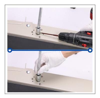
Remove the screw of the connecting rod on the side of the transfer table, and remove the connecting rod.
