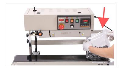
After setting the parameters of the control panel, the bag can be placed under the baffle at the start of sealing to start conveying and then seal. (6) Operation:
