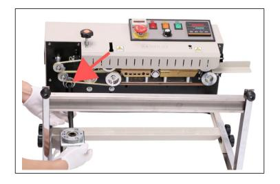
After connecting the bracket to the machine, let the control panel of the machine face up, put the machine down on the ground, and insert the control bar into the round hole as shown in the figure.
