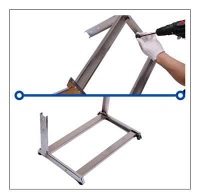
Install the non-slip feet on the bottom of the stand.
