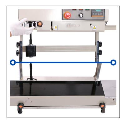
Stabilize the control lever by hand, and slowly put the machine upright.
