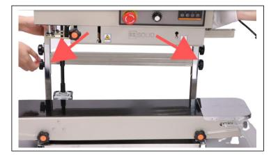
The yellow and black fasteners on both sides of the bracket can adjust the height at the same time to achieve the height suitable for the bag you need to seal.
